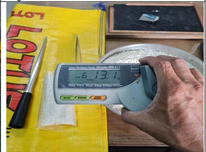
Photo No. 09: Moisture testing
